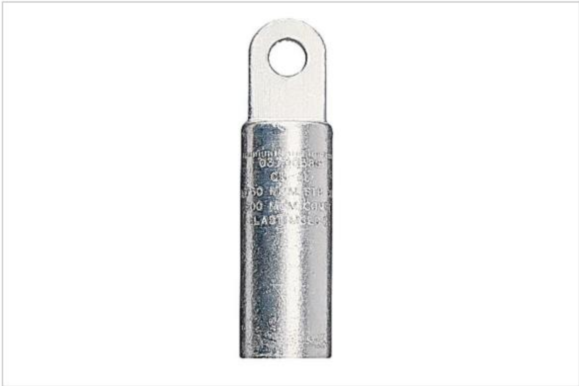
Elastimold 3700270 4/0 Compression Lug 15/25 600Amp Deadbreak 4/0 stranded compressed or 250 compact/solid
